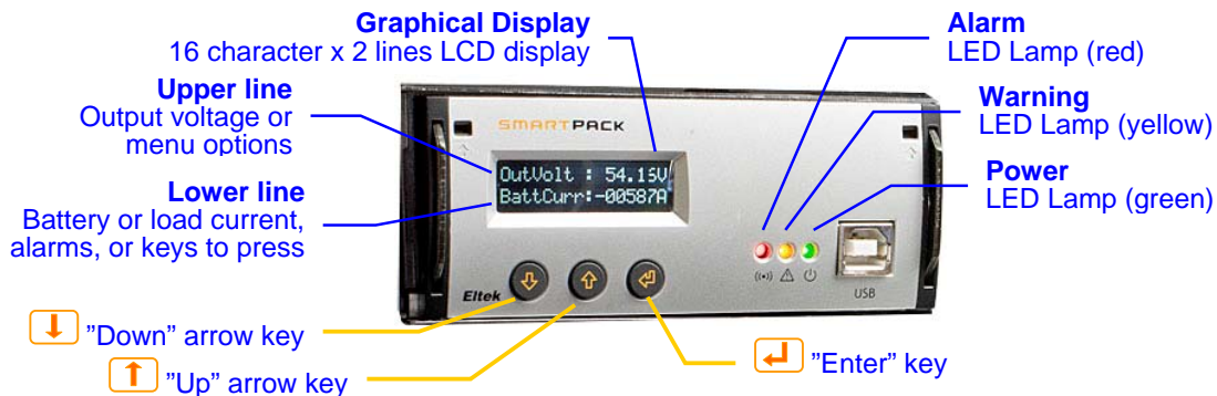
Figure 19 Smartpack controller's front keys and indicators
