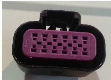
Vehicle side mating connector
