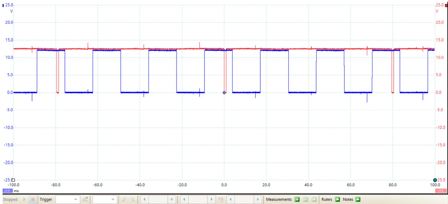
Idling. Blue signal is tacho signal. Red is injection signal. L/100km = 0.
